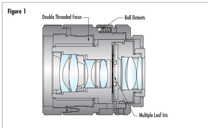
Figure 1: Standard imaging lens with complex mechanics and an adjustable iris
