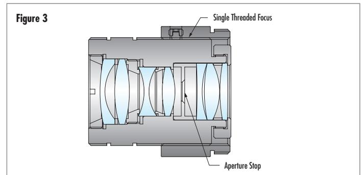
Figure 3: Industrial Ruggedized lens with simplified mechanics
