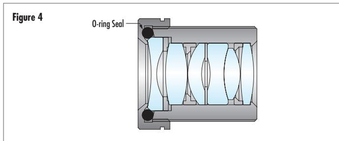
**Figure 4:** Ingress Protection Ruggedized lens with an O-ring to seal out contaminants
