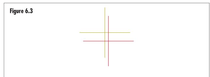
**Figure 6.3:** Image crosshairs overlaid, red crosshair is image from Figure 6.1 and the decentered yellow crosshair is from Figure 6.2. Example is highly exaggerated actual changes tend to be on the order of a pixel or less.
