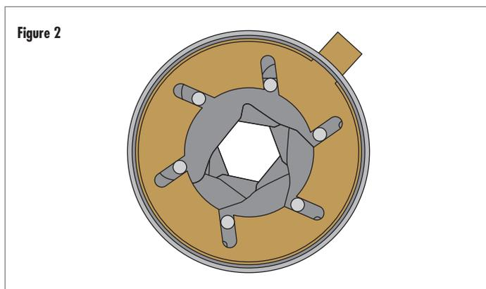
Figure 2: Standard iris with moving leaves
