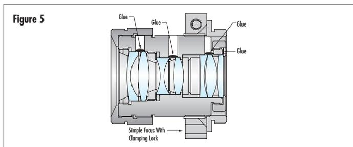
**Figure 5:** Stability Ruggedized lens with all elements glued in place
