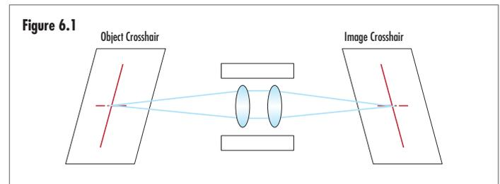
**Figure 6.1:** Unperturbed system where object crosshair is mapped to the image crosshair
