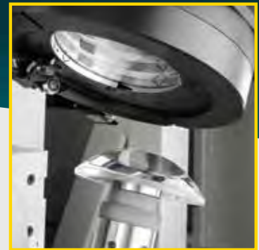
QED ASI™ Aspheric Stitching Interferometer
