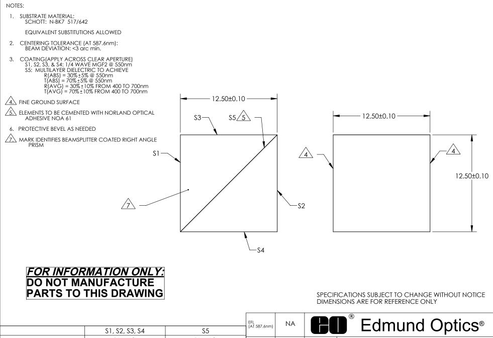
SHAPE **PLANO** PLANO 12.5mm 30R/70T Standard Cube Beamsplitter BFL NA TITLE 1/4 WAVE 1/4 WAVE SURFACE ACCURACY AT 632.8nm (P-V) (AT 587.6nm) 60 - 40 60 - 40 SURFACE QUALITY SHEET DWG NO 68548 ALL DIMS IN mm MIN CLEAR APERTURE 11.5 x 11.5mm 17.6 x 11.5mm 1 OF 1
