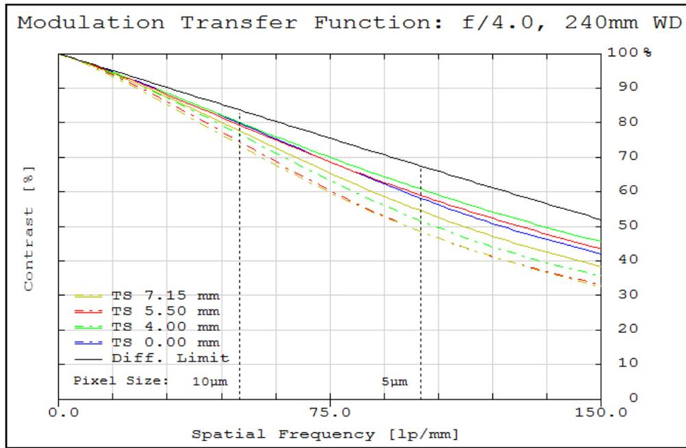
**Figure 3:** Image space polychromatic diffraction FFT Modulation Transfer Function (MTF) for  $\lambda = 486\text{nm}$  to  $656\text{nm}$ . Included are Tangential and Sagittal values for field points on center, at 70% of full field and at the maximum sensor format. Solid black line indicates diffraction limit determined by  $f/\#$ -defined aperture. Frequencies corresponding to the Nyquist resolution limit of pixel sizes are indicated.
