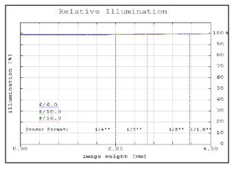
Figure 2: Relative illumination (center to corner)
