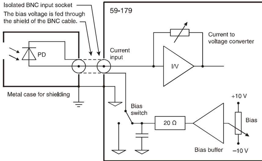
Photo detector biasing through external voltage source
