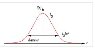
Figure 1. The spot size is usually defined as the radial distance from the center point of maximum irradiance to point where the intensity drops to 1/e<sup>2</sup> of the initial value.
