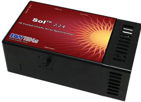
The Sol™ 2.2A is a high performance linear InGaAs array spectrometer featuring 256 pixels and providing high throughput and large dynamic range with TE cooling down to -15°C via a built-in 3-stage cooler.
