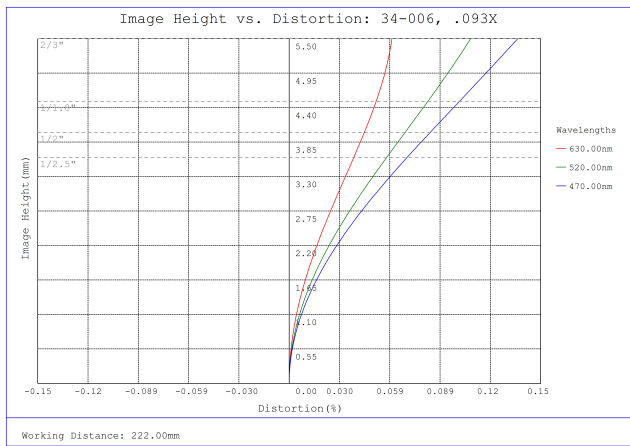
#34-006, 0.093X, 2/3" C-Mount TitanTL® Telecentric Lens, Distortion Plot
