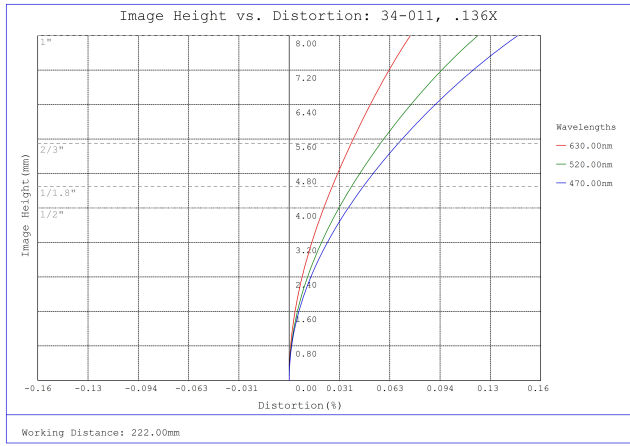
#34-011, 0.136X, 1" C-Mount TitanTL® Telecentric Lens, Distortion Plot
