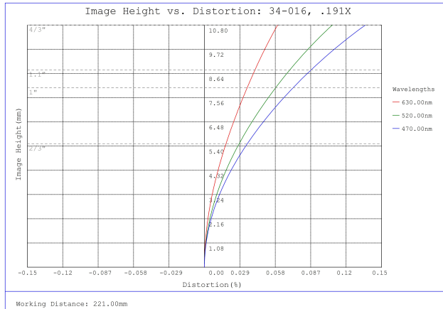
#34-016, 0.191X, 4/3" C-Mount TitanTL® Telecentric Lens, Distortion Plot
