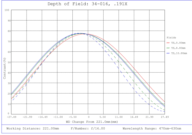
#34-016, 0.191X, 4/3" C-Mount TitanTL® Telecentric Lens, Depth of Field Plot, 221mm Working Distance, f16
