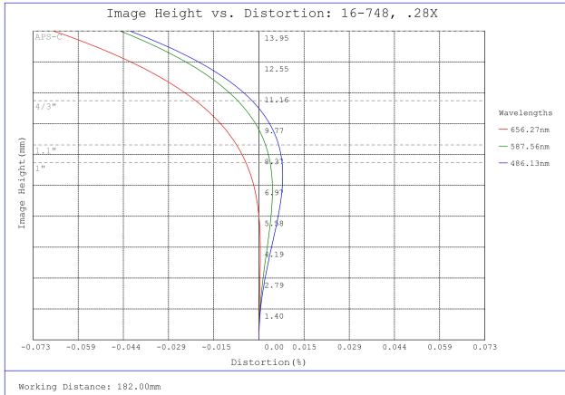
#16-748, 0.28X, 28.7mm TFL-Mount PlatinumTL™ Telecentric Lens, Distortion Plot
