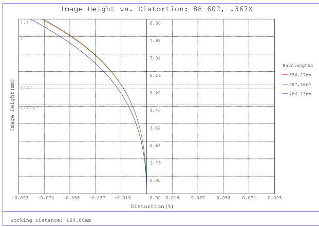
#88-602, 0.367X CobaltTL Telecentric Lens, Distortion Plot
