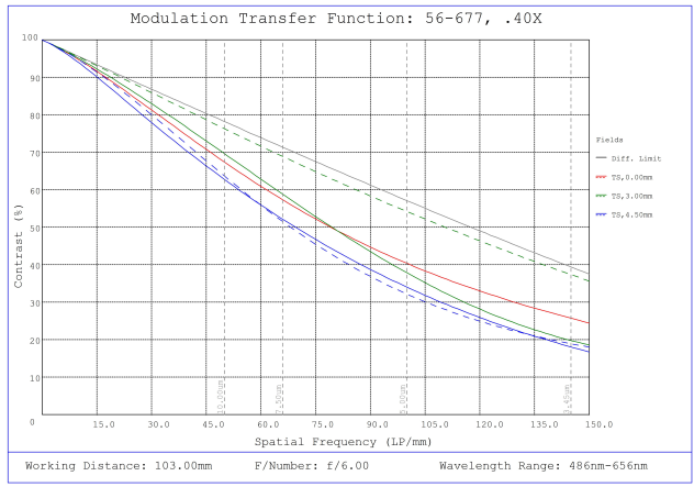
#56-677, 0.40X SilverTL™ Telecentric Lens, Modulated Transfer Function (MTF) Plot, 103mm Working Distance, f6
