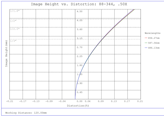
#88-344, 0.50X In-Line Illumination SilverTL™ Telecentric Lens, Distortion Plot
