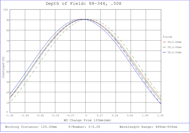
#88-344, 0.50X In-Line Illumination SilverTL™ Telecentric Lens, Depth of Field Plot, 120mm Working Distance, f6
