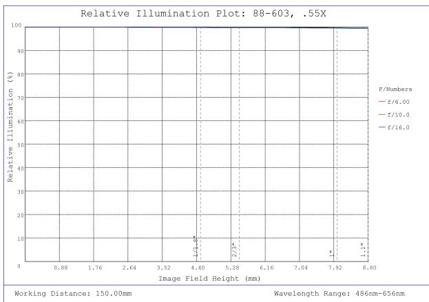
#88-603, 0.55X CobaltTL Telecentric Lens, Relative Illumination Plot
