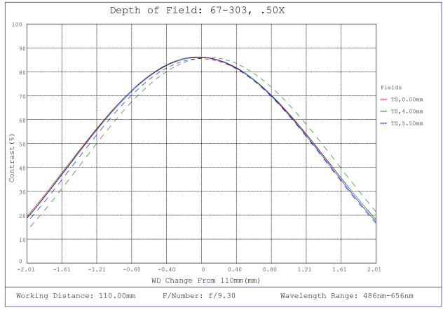
#67-303, 0.5X, 110mm WD, In-Line CompactTL™ Telecentric Lens, Modulated Transfer Function (MTF) Plot, 110mm Working Distance, f9.3
