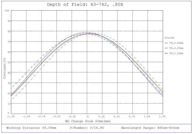
#63-742, 0.8X, 65mm WD CompactTL™ Telecentric Lens, Modulated Transfer Function (MTF) Plot, 65mm Working Distance, f14.9
