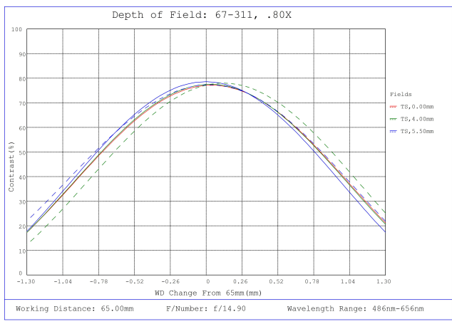
#67-311, 0.8X, 65mm WD, In-Line CompactTL™ Telecentric Lens, Depth of Field Plot, 65mm Working Distance, f14.9
