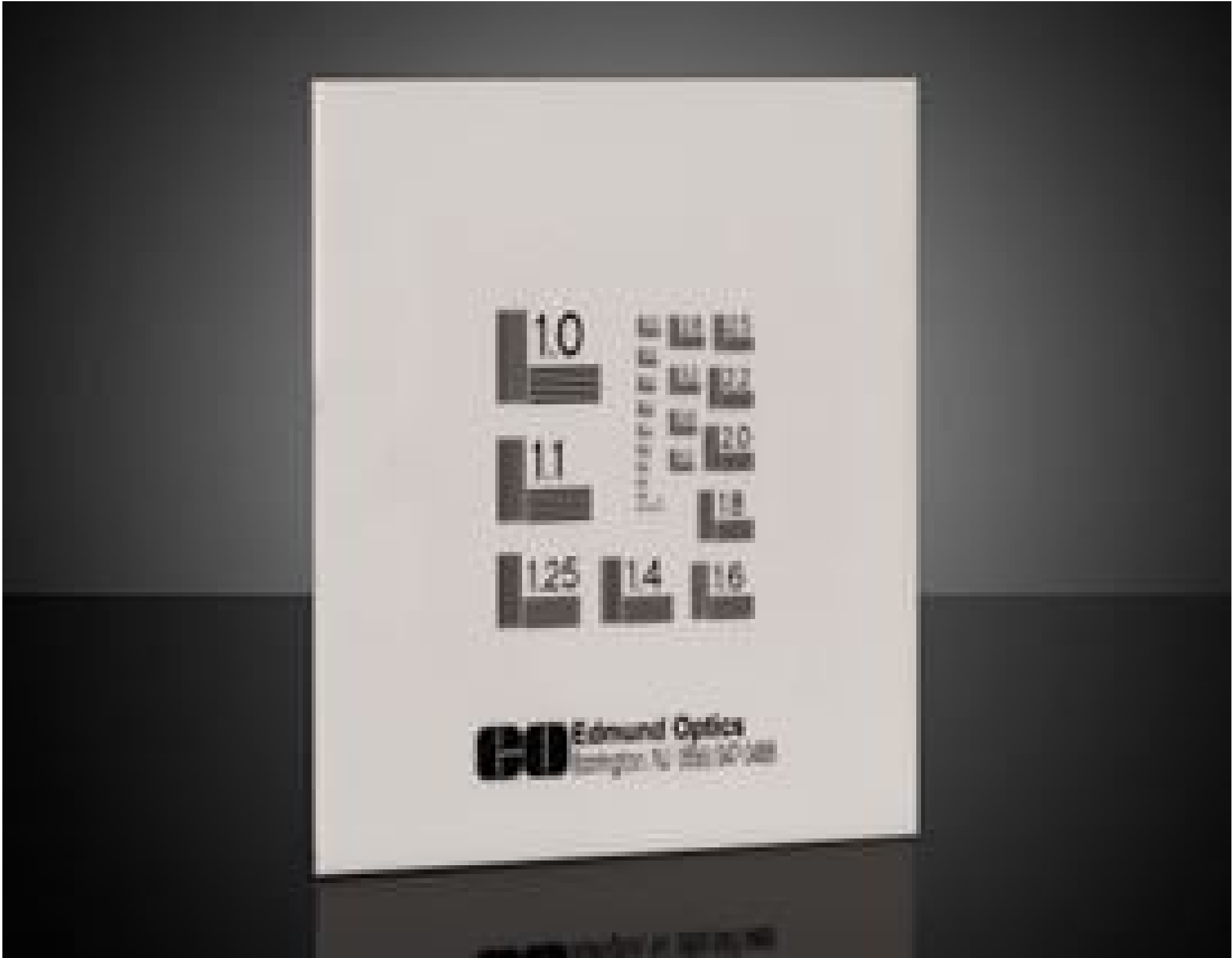
NBS 1963A Resolution Target
