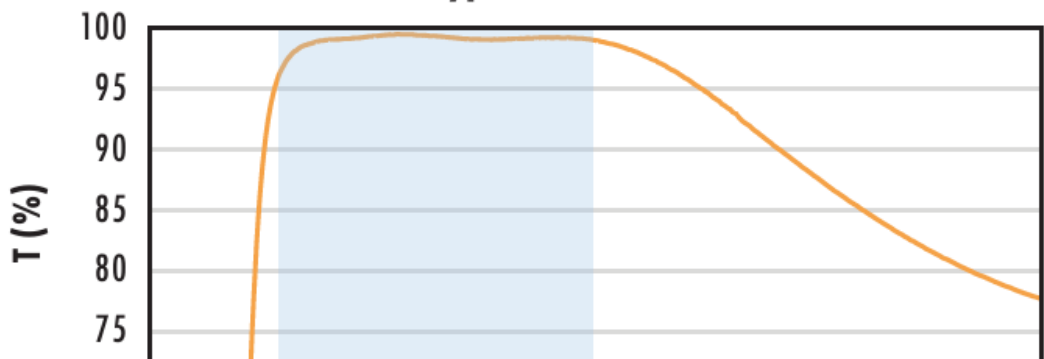
N-BK7 with VIS-EXT Coating Typical Transmission
