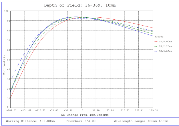
#36-369, 10mm FL f/4, Rugged Blue Series M12 Lens, Depth of Field Plot, 400mm Working Distance, f4
