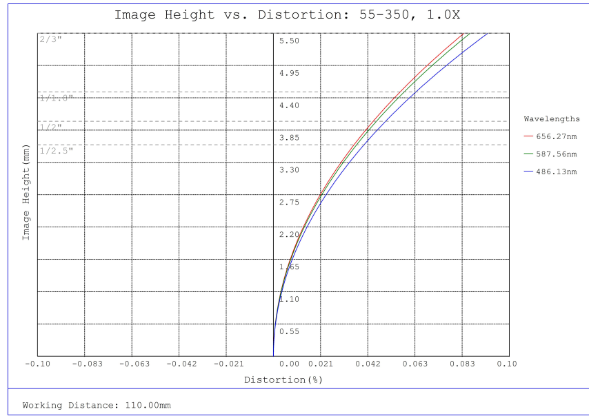
#55-350, 1.0X 2/3" GoldTL™ Telecentric Lens, Distortion Plot
