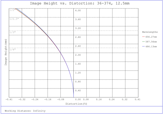
#36-374, 12.5mm FL f/5.6, Rugged Blue Series M12 Lens, Distortion Plot
