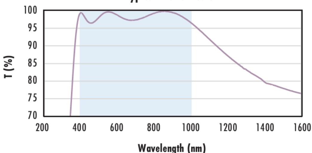
Typical transmission of a 3mm thick N-BK7 window with MS-NIR (400-1000nm) coating at 0° AOI.
