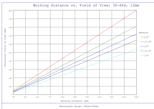
#36-864, 12mm f/11, 1000mm-∞ Primary WD, HRr Series Fixed Focal Length Lens, Working Distance versus Field of View Plot
