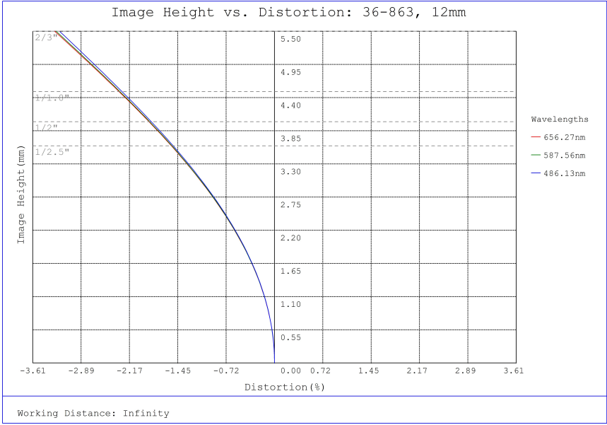
#36-863, 12mm f/11, 400-2000mm Primary WD, HRr Series Fixed Focal Length Lens, Distortion Plot
