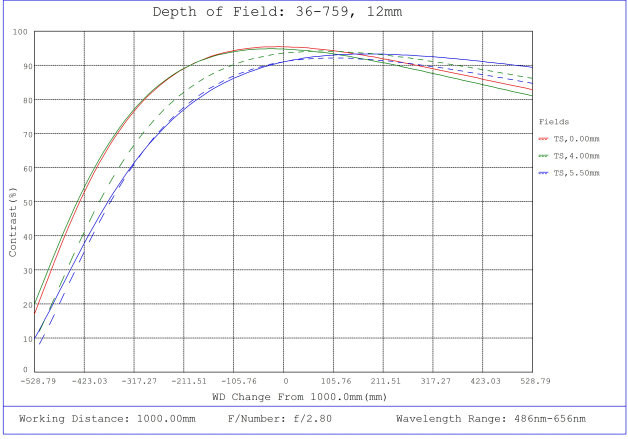
#36-759, 12mm f/2.8, 1000mm-∞ Primary WD, HRI Series Fixed Focal Length Lens, Depth of Field Plot, 1000mm Working Distance, f2.8
