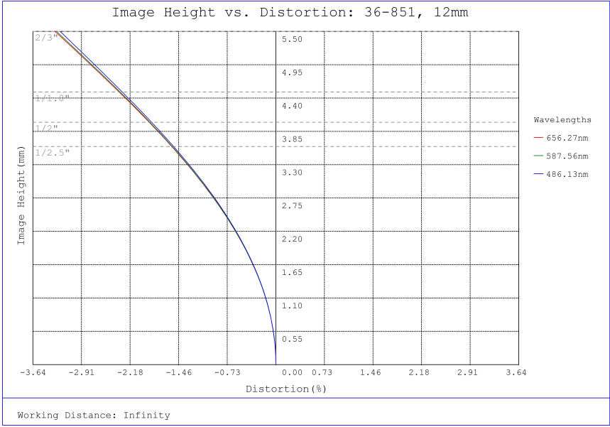
#36-851, 12mm f/2.8, 1000mm-∞ Primary WD, HRr Series Fixed Focal Length Lens, Distortion Plot
