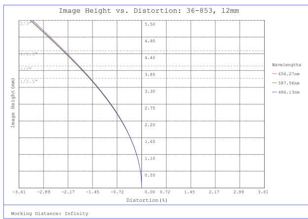
#36-853, 12mm f/4, 400-2000mm Primary WD, HRr Series Fixed Focal Length Lens, Distortion Plot
