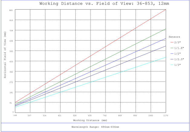
#36-853, 12mm f/4, 400-2000mm Primary WD, HRr Series Fixed Focal Length Lens, Working Distance versus Field of View Plot
