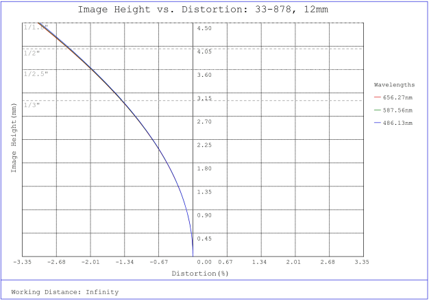
#33-878, 12mm, f/4 UCi Series Fixed Focal Length Lens, Distortion Plot
