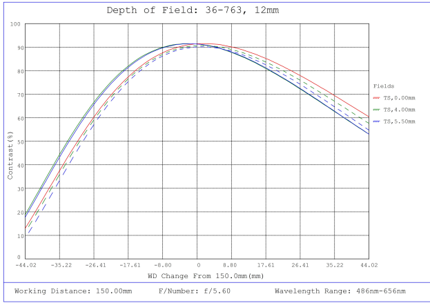
#36-763, 12mm f/5.6, 150-500mm Primary WD, HRI Series Fixed Focal Length Lens, Depth of Field Plot, 150mm Working Distance, f5.6
