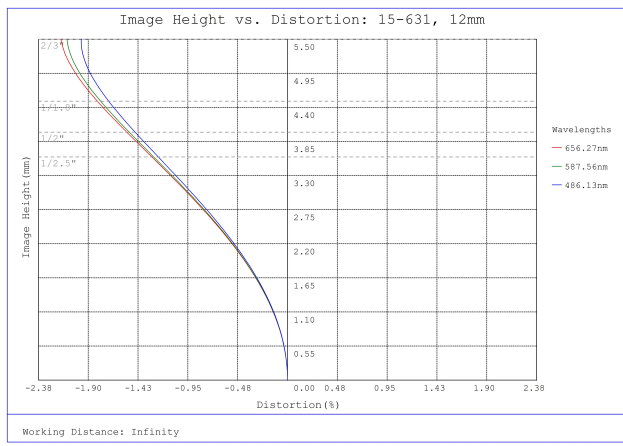
#15-631, 12mm, f/1.8 Cw Series Fixed Focal Length Lens, Distortion Plot
