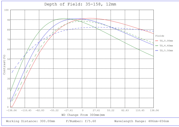
#35-158, 12mm, f/5.6 Cr Series Fixed Focal Length Lens, Depth of Field Plot, 300mm Working Distance, f5.6
