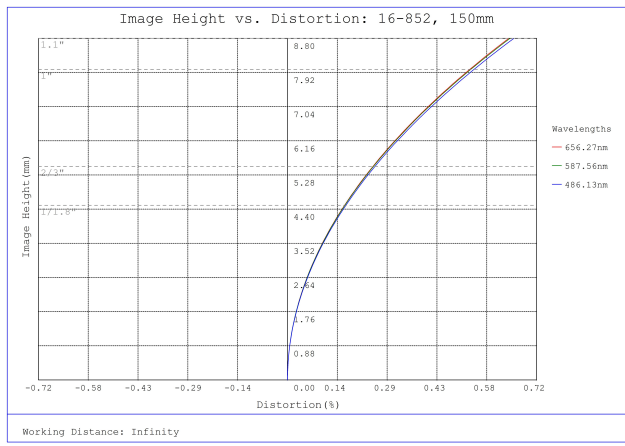
#16-852, 150mm, f/4 Athermal Lens, Distortion Plot
