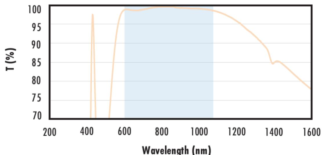
Typical transmission of a 3mm thick fused silica window with NIR I (600 - 1050nm) coating at 0° AOI.
