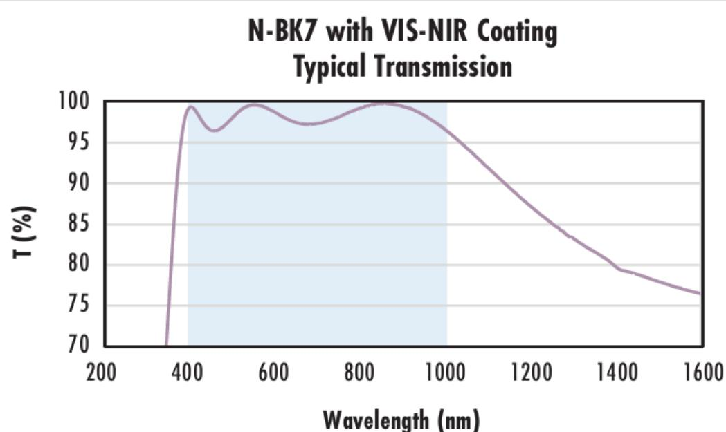
Typical transmission of a 3mm thick N-BK7 window with VIS-NIR (400-1000nm) coating at 0° AOI.
