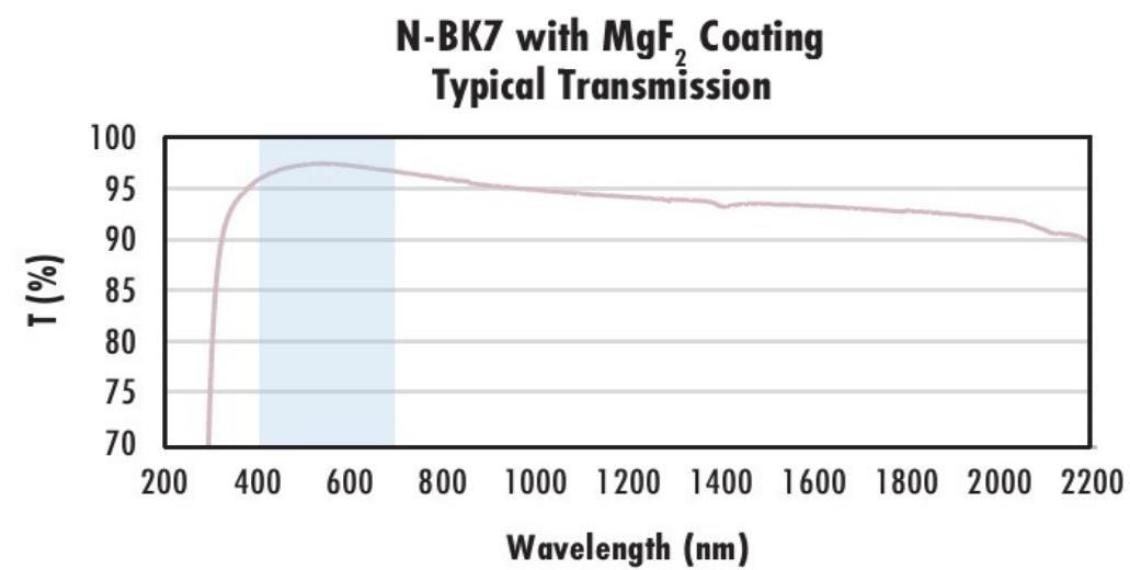
Typical transmission of a 3mm thick N-BK7 window with MgF2 (400-700nm) coating at 0° AOI.
