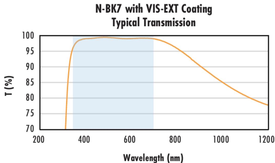
Typical transmission of a 3mm thick N-BK7 window with VIS-EXT (350-700nm) coating at 0° AOI.
