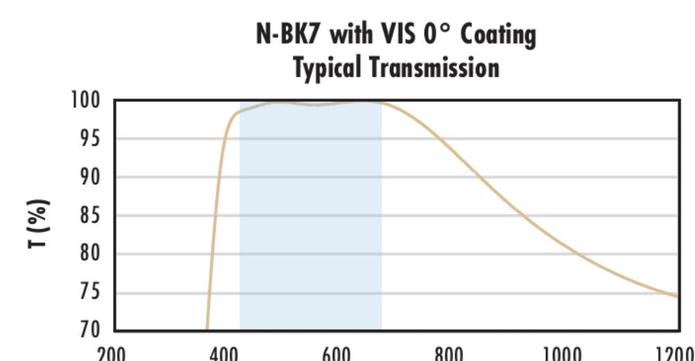
Typical transmission of a 3mm thick N-BK7 window with VIS 0° (425-675nm) coating at 0° AOI.
