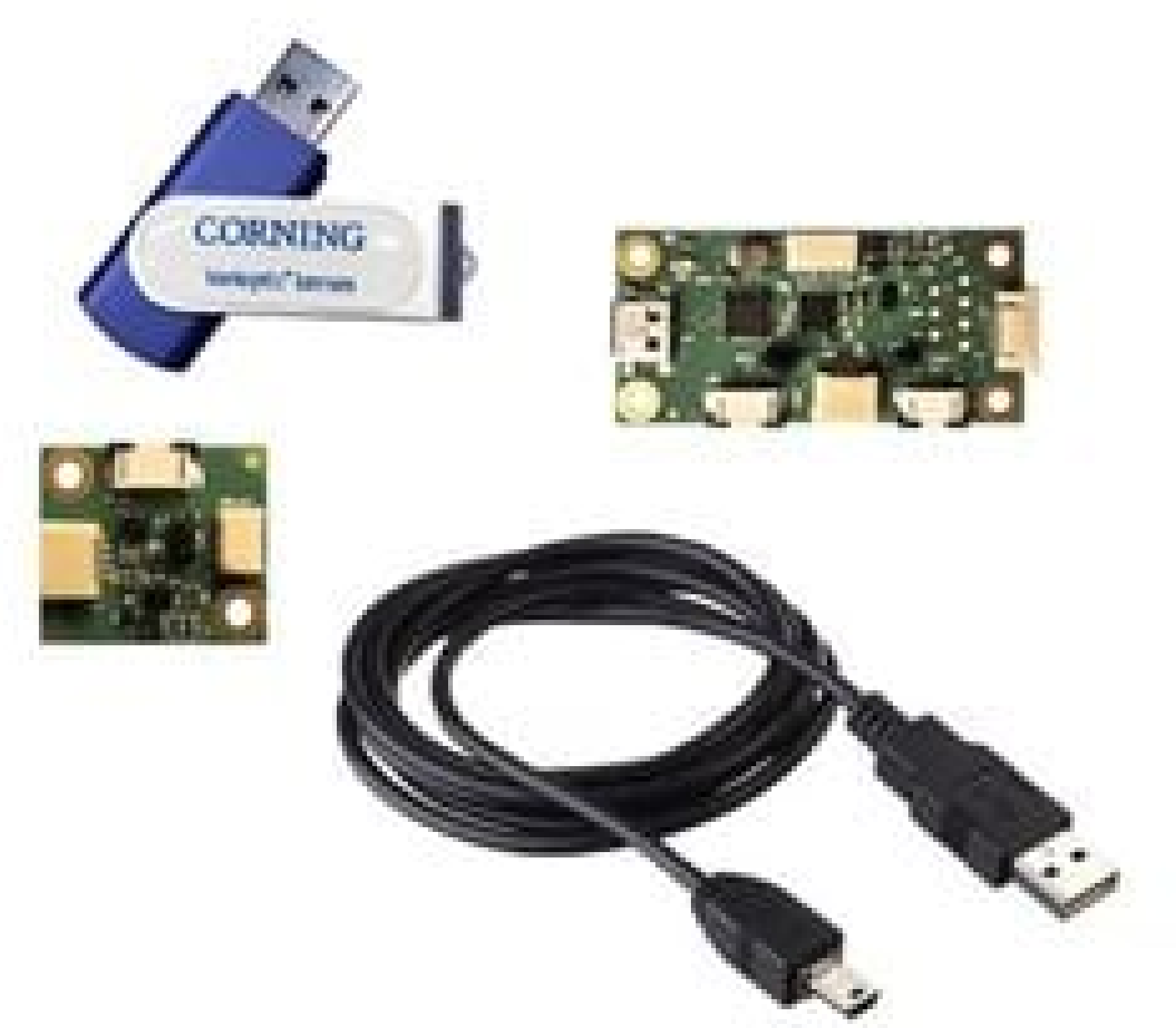
1.6mm CA, Corning® Varioptic® Variable Focus Liquid Lens Development Kit (Included Electronics)
