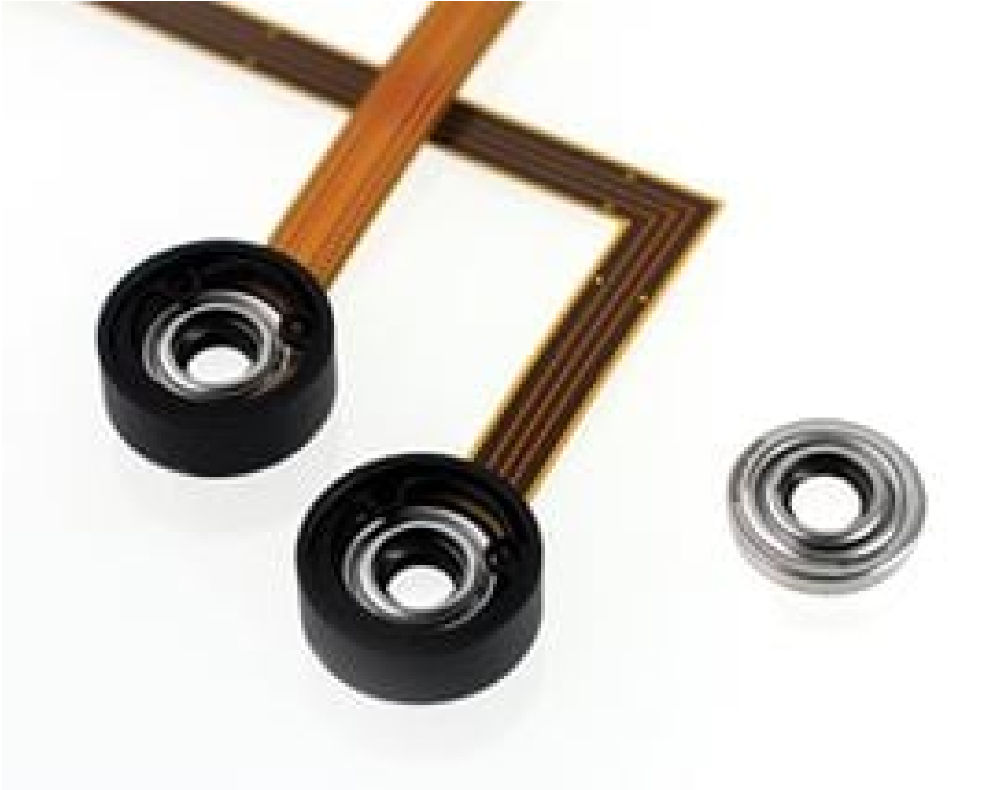
Corning® Varioptic® Variable Focus Liquid Lenses
