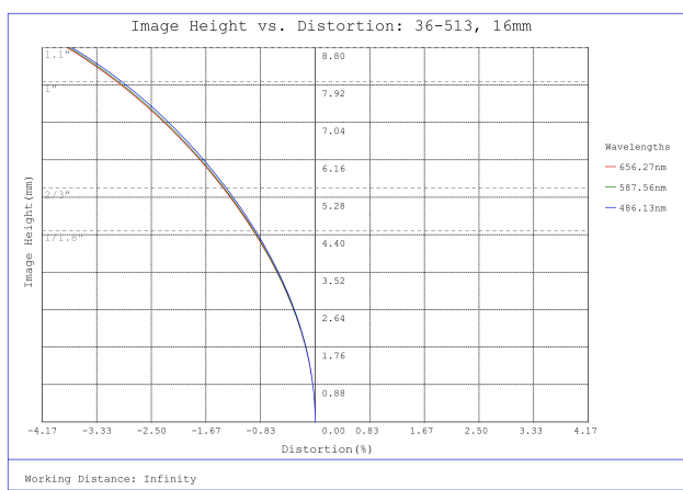
#36-513, 16mm f/4, HPr Series Fixed Focal Length Lens, Distortion Plot
