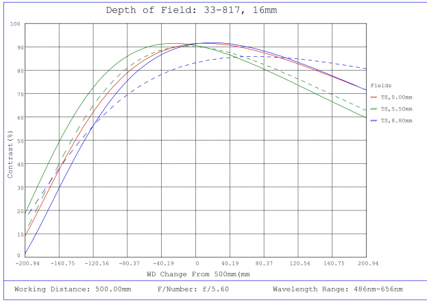
#33-817, 16mm f/5.6, HPI Series Fixed Focal Length Lens, Depth of Field Plot, 500mm Working Distance, f5.6
