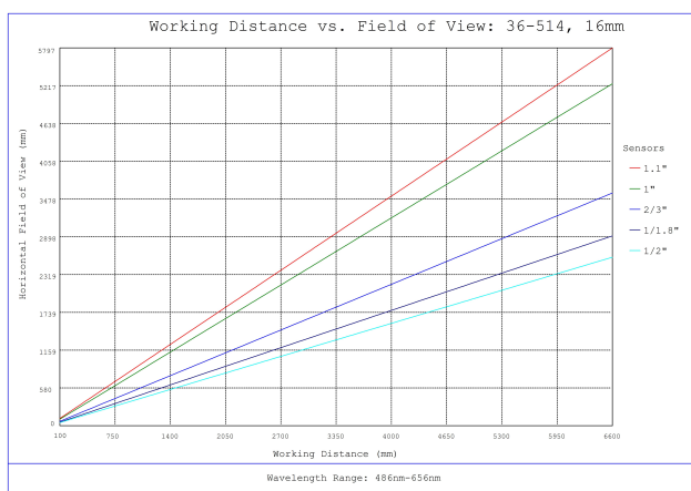
#36-514, 16mm f/5.6, HPr Series Fixed Focal Length Lens, Working Distance versus Field of View Plot
