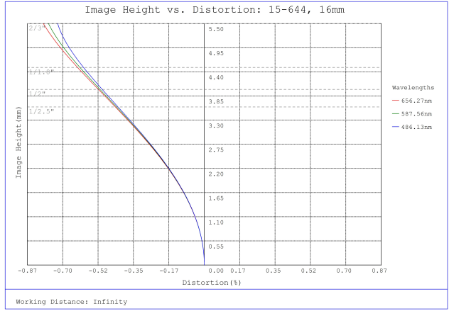
#15-644, 16mm, f/11 Cw Series Fixed Focal Length Lens, Distortion Plot
