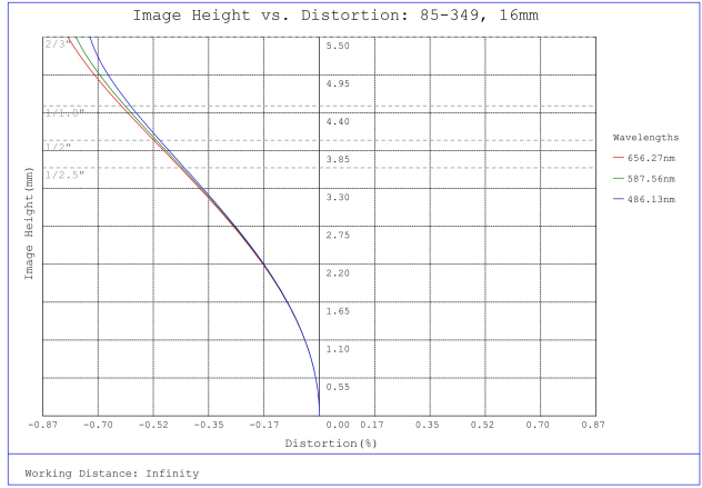
#85-349, 16mm, f/1.8 Ci Series Fixed Focal Length Lens, Distortion Plot
