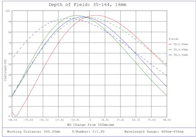
#35-164, 16mm, f/1.8 Cr Series Fixed Focal Length Lens, Depth of Field Plot, 500mm Working Distance, f1.8
