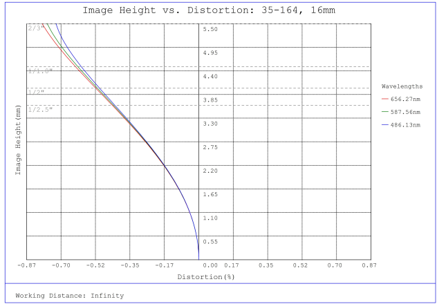
#35-164, 16mm, f/1.8 Cr Series Fixed Focal Length Lens, Distortion Plot
