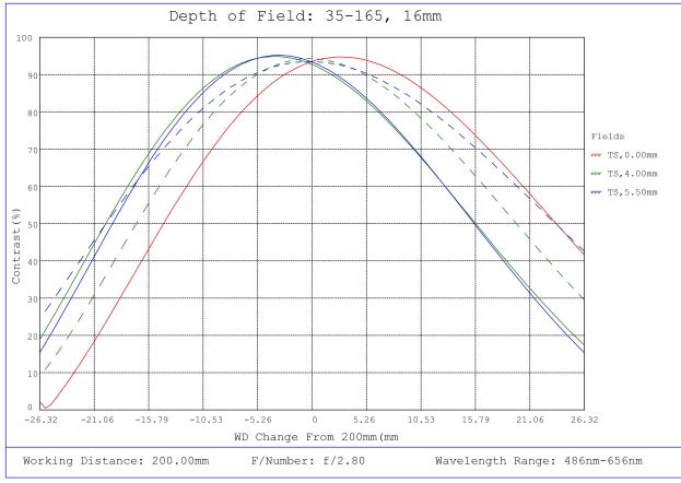
#35-165, 16mm, f/2.8 Cr Series Fixed Focal Length Lens, Depth of Field Plot, 200mm Working Distance, f2.8
