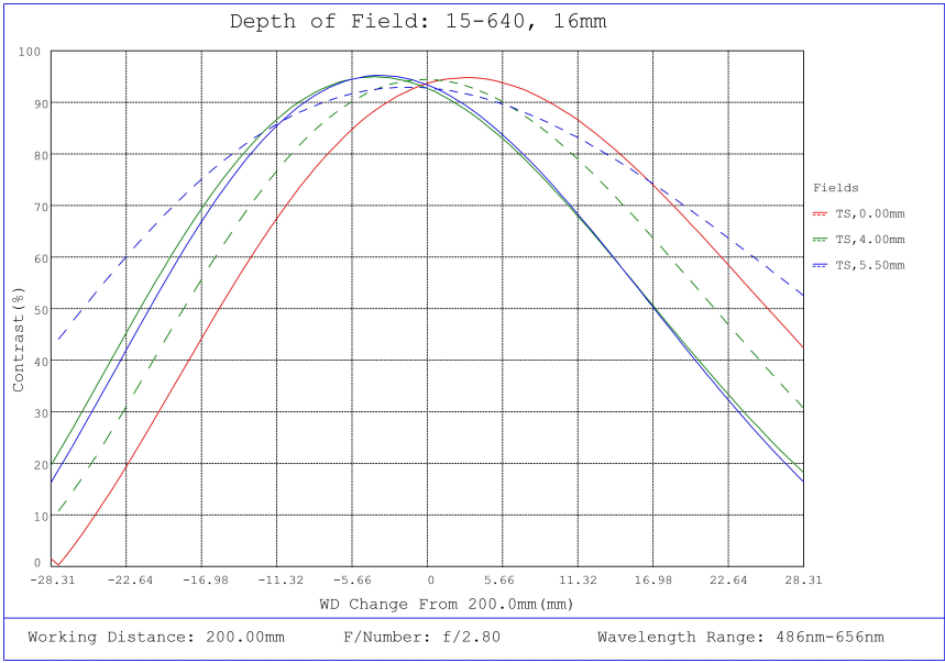
#15-640, 16mm, f/2.8 Cw Series Fixed Focal Length Lens, Depth of Field Plot, 200mm Working Distance, f2.8
