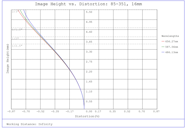
#85-351, 16mm, f/4 Ci Series Fixed Focal Length Lens, Distortion Plot
